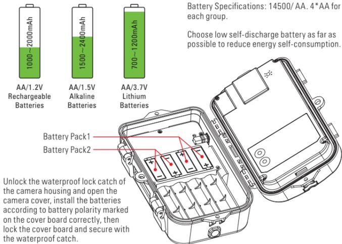
Unlock the waterproof lock catch of the camera housing and open the camera cover, install the batteries according to battery polarity marked on the cover board correctly, then lock the cover board and secure with the waterproof catch.
